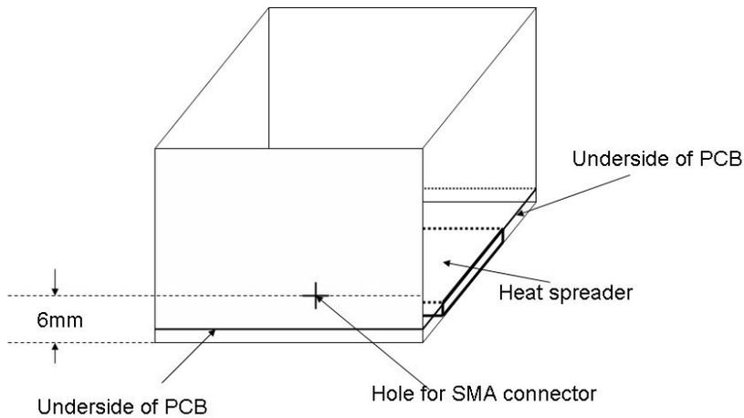
**Use only M2.5 pan head screws, do not use washers, do not be tempted to drill the holes bigger and use M3 or the heads will short to the matching lines.** Bolt the assembled board and heat spreader to a large heatsink
