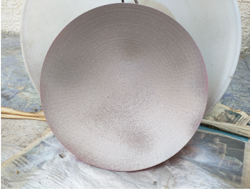
Dish after one coat of conductive spray paint. You can still see a haze of Hello Kitty 15 pink.
