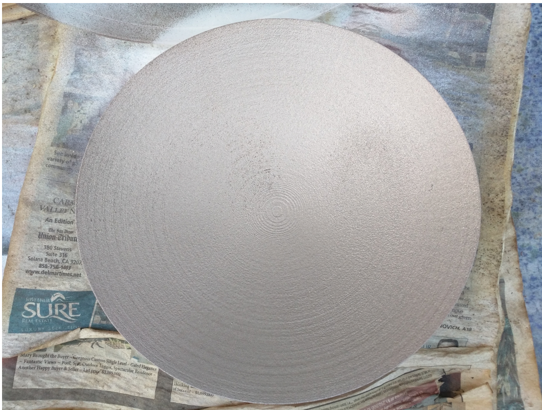
Dish after two coats of conductive spray paint. Coverage improved!
