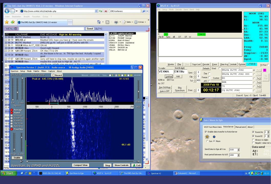
This is the 529 CW-signal (R OOO) from W5LUA in a QSO with VE4MA at 17.2.08. Received with a 2.4m segment dish (f/D 0.33), feed system is a 8mm round wave guide, preamp DB6NT LNA243 RX2 with 1.05dB NF @ -5deg. C. sun noise 10.42dB /moonnoise 1.05 dB
