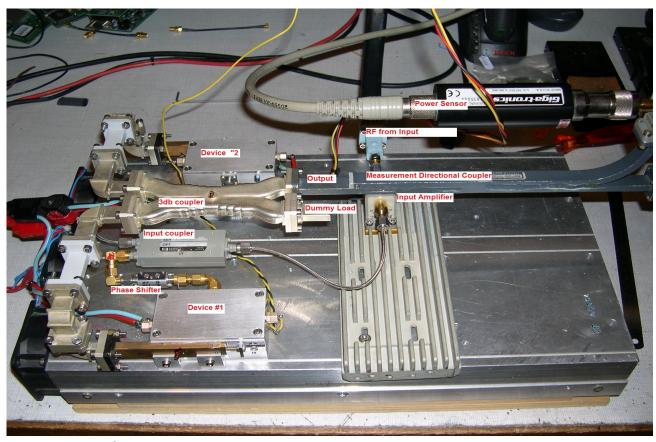
The reasonable performances achieved are more than 15 Watts (41.5 dBm) at the saturation, for approximatively 340 mW (~25 dBm) at the input. Each TGA needs 21 to 22 dBm in, plus the insertion losses in each input branch which are around 2.5db (insertion loss is in addition to 3 dB coupling loss).
