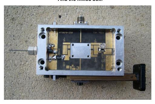
The mechanical drawings of the milled box are provided on the DVD so if you have your own milling machine tool or access to a numerical machine you could reproduce it quite easily.
