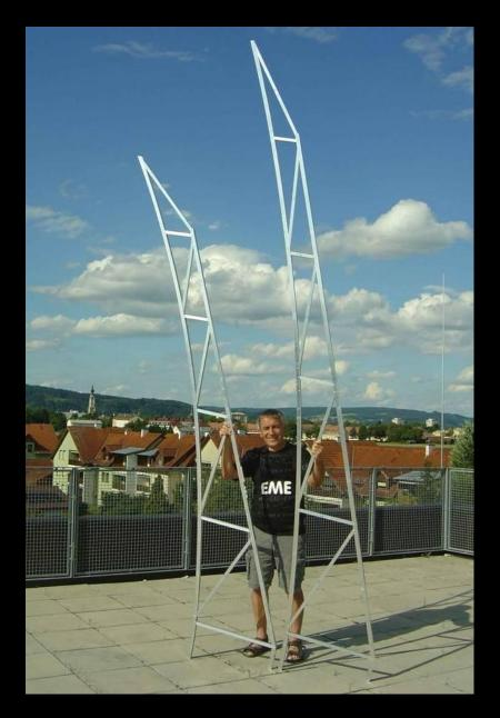
Here you can see an example for the different length and shape of the ribs for my 7.3m dish. The template must be modified after building a pair of ribs every time. Those extra hours of work were only a small fraction of the time I spent for realizing the whole project.
