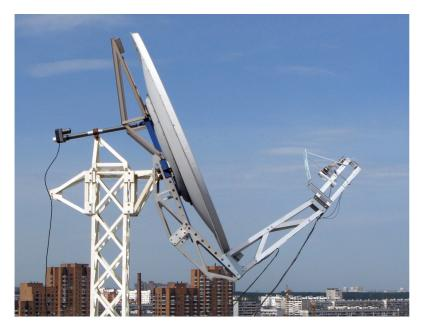
"Supral" company. Antenna 2.4m. diameter is First antenna test on 76 GHz was made in October 2006. These preliminary were attempts to measure the Sun noise. However I actively started to work with antenna only in late 2010, after it was possible to place the beacon in 900 meters away from my house.
