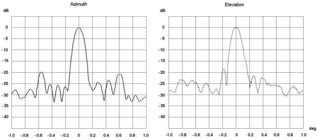
There was a significant improvement of the pattern and about 0.4 dB rise of the antenna gain. It was hard to say whether it's high or low rise. To evaluate the effectiveness of the lens one need to know the scale of the problem. We need to know the difference in gain of my non-ideal antenna and the antenna with an ideal shape of the reflector.
