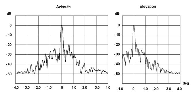
So, we have the data to analyze a part of the radiation pattern, adjacent to the main lobe. From the most common considerations it is clear that smooth deviations from the ideal shape of the dish affecting only this part of the pattern. Based on these diagrams the three-dimensional pattern of the antenna was built for two cases - with and without the lens. The integration of 3D pattern gives the following results.
