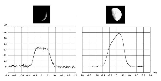
Moon noise on 77 GHz is strongly depends on the phase of the Moon. The noise level of the full Moon is about two times higher than of the new Moon. In contrast to the lower frequency bands, you cannot find the center of the moon by the noise maximum, and need to be guided by the edge of the lunar disk.
