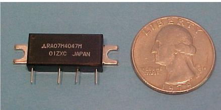
Figure 1. The 7 Watt RA07M4047M and a Quarter
