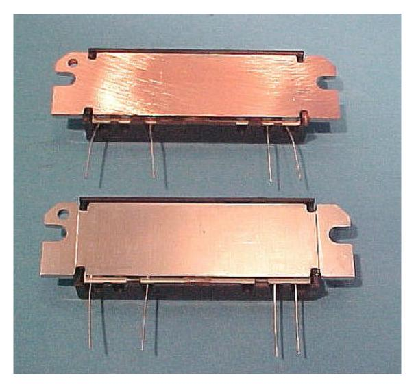
The surface is as smooth as the original M57762. It is very simple to do but care must be taken not to over heat the hybrid. Copper conducts heat fast! To eliminate the amount of inductance from the bypass capacitors to the flange, a few further steps have been performed. The important things to notice are the shield and the extra mounting screw between the gate and drain voltage pins.
