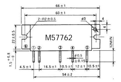
Figure 2. Physical dimensions of modules.
