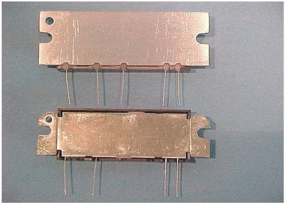
The mounting precautions went into detail of how flat the heat sink should be to expect the best performance so I didn't expect to see the "Flange" and I over looked it on the data sheet.
