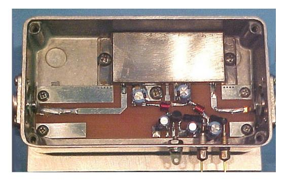
In combination, the screw holds the bottom of the PCB down to the heat sink to ensure the shortest path of the by-pass capacitors to modified flange of he hybrid. The addition of the shield after it is soldered to the ground connections on the PC board is to now reduce the inductance even further. This design is now unconditionally stable and ready for the RF test.
