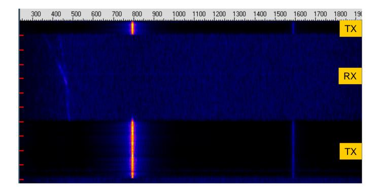
ON4IY 1296 MHz 750 mW 360 km recorded in NAC May 2006 (each red tick is 10 seconds): just readable in CW in the peak
