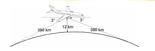
Haximum range by airplane at FL400 at the right position and radio LOS path including refraction in the atmosphere is 1040 km
