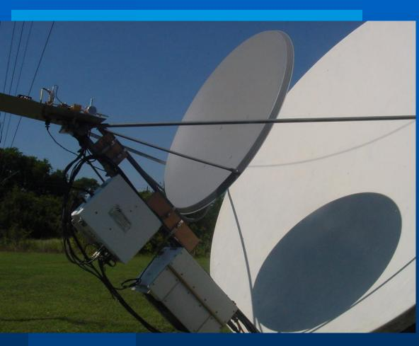
Tests on 2.4 m & **1m Dishes** Best Results from a 1m TV minidish •7 dB Sun Noise, 0.75 dB Moon Noise •50 Ohm/ Cold Sky 1.2 dB Ta = 133 KStill Room to **Optimize**
