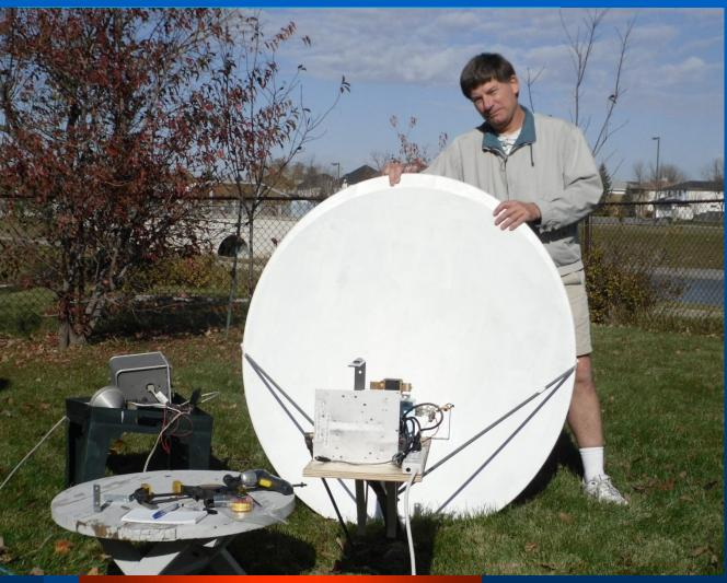
Best Results from a 1.2m **Satellite dish** •4.8 dB Sun Noise, still 6.1 dB NF Dish was old Hughes **DirecWay** "KA" dish with aluminum foil added
