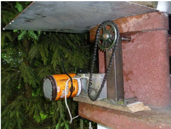
It was really a wet day. I had to protect the drive, which was constructed by Helmut from his daughters bicycle and a motor from an old "Siemens Oszillereg, against rain!
