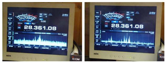
Next both pictures are showing the signal from DL0GTH. Note that their signal is even some dB stronger but the noise- floor is nearly 30dB less! I know that my homemade transverter is not perfect, but the comparison between both signals with nearly the same signal- strength shows that the noise- floor on the spectrum- display from my IC7700 is not produced by my own local oscillator.
