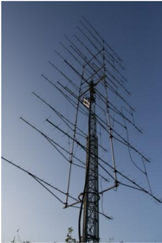
The antennas for 2m, 13cm and 3cm, 2m and 23cm, the monster for 70cm and 6m with 2m vertical
