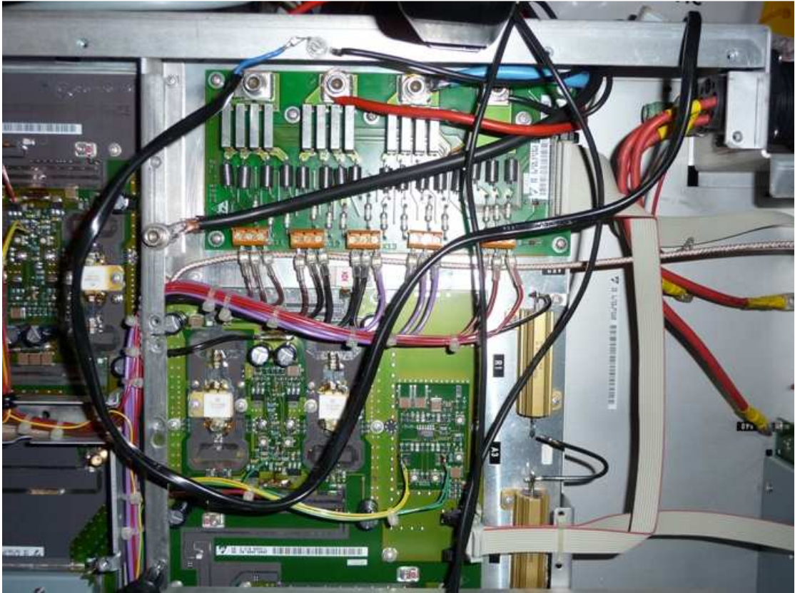
The temporary connection of the power- supplies to the amplifier.
