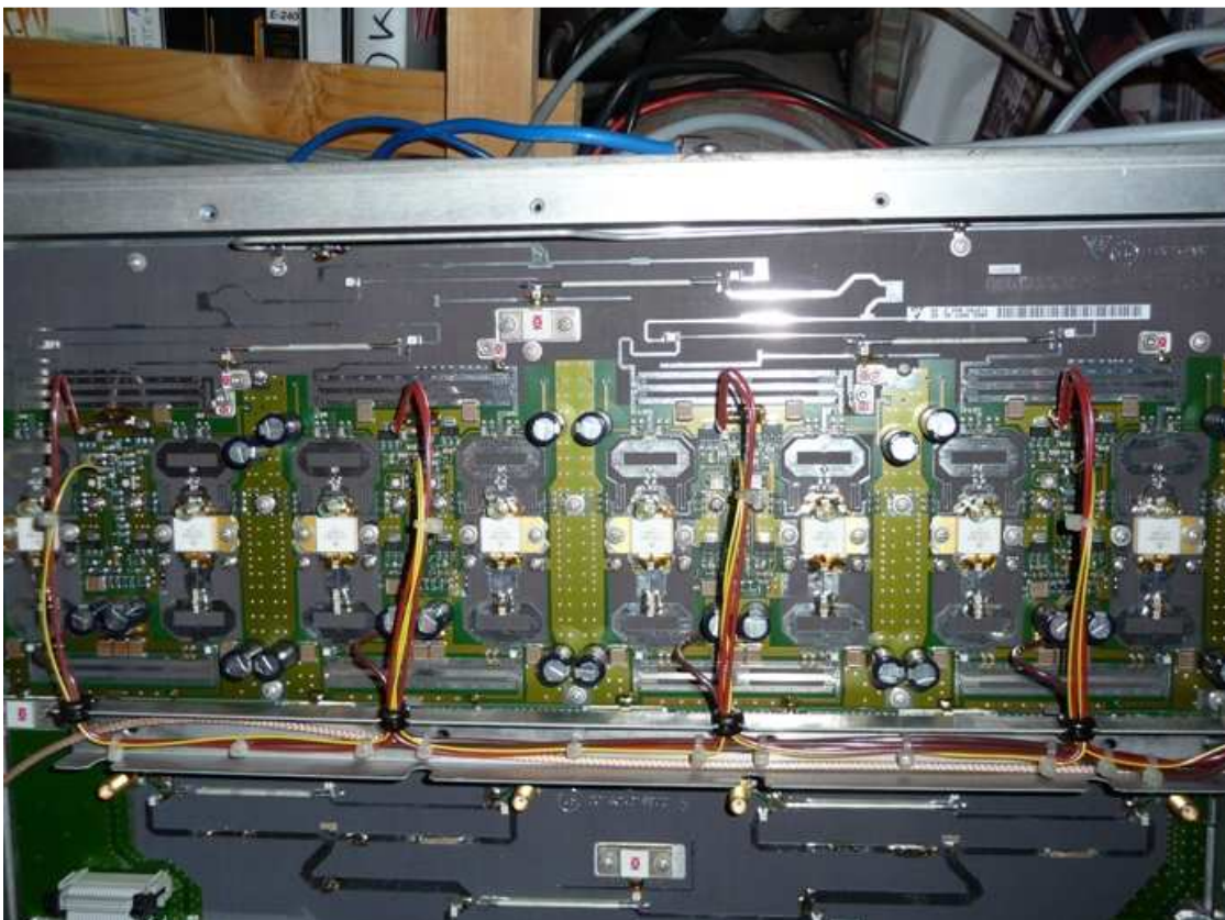
This picture shows the half part of the final amplifier after doing some modifications.
