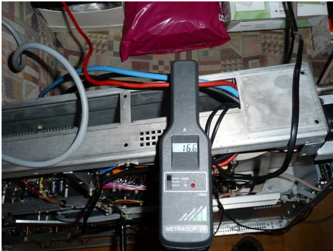
This picture shows the current for the pre- and driver with driving power from about 3Watts.
