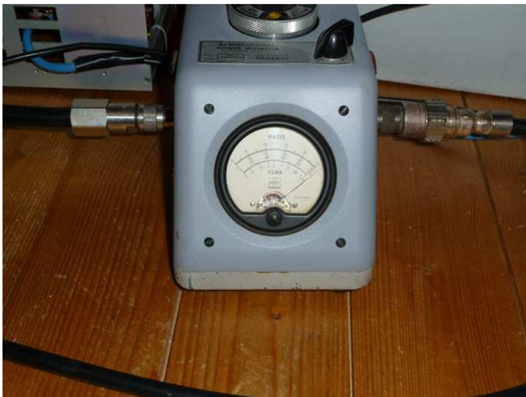
End of scale of the power- meter. 1KW power output can be very easy reached with 3W driving power!
