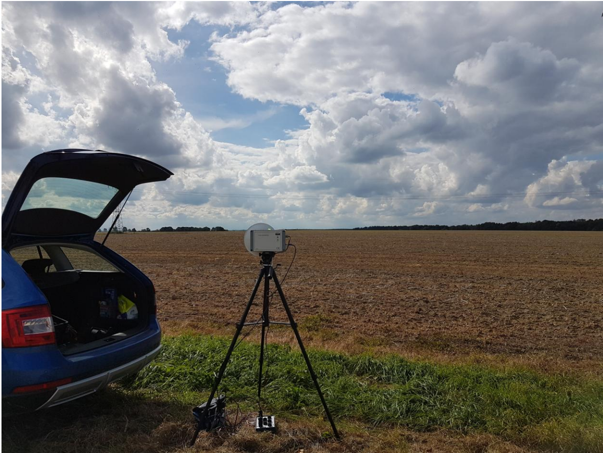
DL6NCI in JO61BA, 250m ASL near the city of Zeitz 47GHz: 1W out 25cm dish
