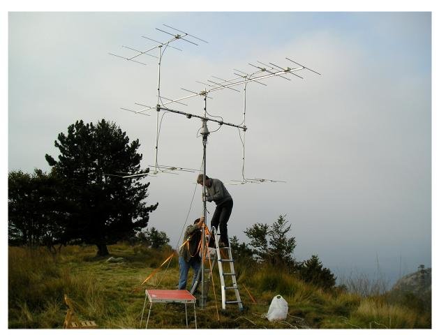
working with the amazing Rob (BPU) equipment. We assembled four five-elements antenna DK7ZB and one nine-elements DK7ZB, home made by Dado (NRI), rtx 2mt., amplifier, bird, rotor, power generator, table, chairs, etc,.... At 9.30 AM we were on air with 200 W and we started the calls.
