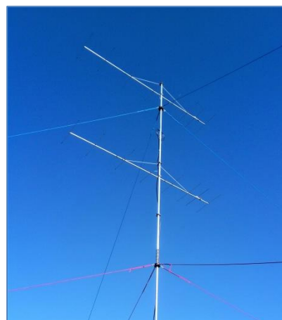
The 2x8 element DK7ZB antenna system in the Sunday morning sun
