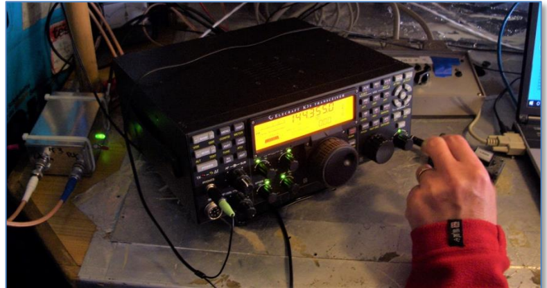
The K3s transceiver in action on our calling frequency. At the left side the IF crystal filter box
