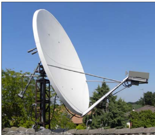
Pictures: Left: 24 GHz experimental feeds which allow for a greater gain on my offset dish compared to a W2IMU 1.8 wl – Middle: Picture B: Search for optimal opening on E and H plane and flare length of new feeds with WR42 WG – Right: 10 & 24 GHz Feeds. With the 10GHz feed installed on 2.7 m dish I measured 18 dB sun noise with SFU 135.7. I have calculated 50 dBi dish gain.
