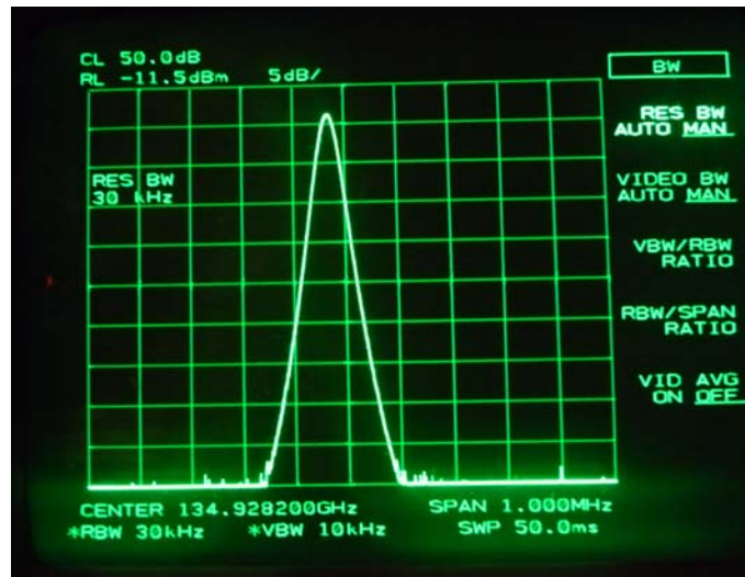
Fig. 12: The 134.928 GHz signal on the analyser
