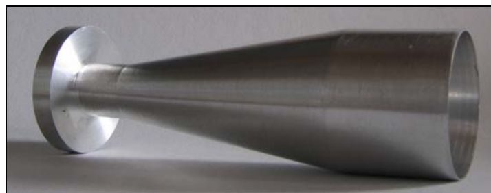
Fig. 13: Horn for 122 GHz, photo by Bert, PE1RKI
