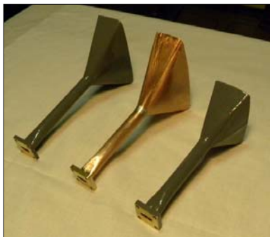
Pictures: Left: 24 GHz experimental feeds which allow for a greater gain on my offset dish compared to a W2IMU 1.8 wl – Middle: Picture B: Search for optimal opening on E and H plane and flare length of new feeds with WR42 WG – Right: 10 & 24 GHz Feeds. With the 10GHz feed installed on 2.7 m dish I measured 18 dB sun noise with SFU 135.7. I have calculated 50 dBi dish gain.
