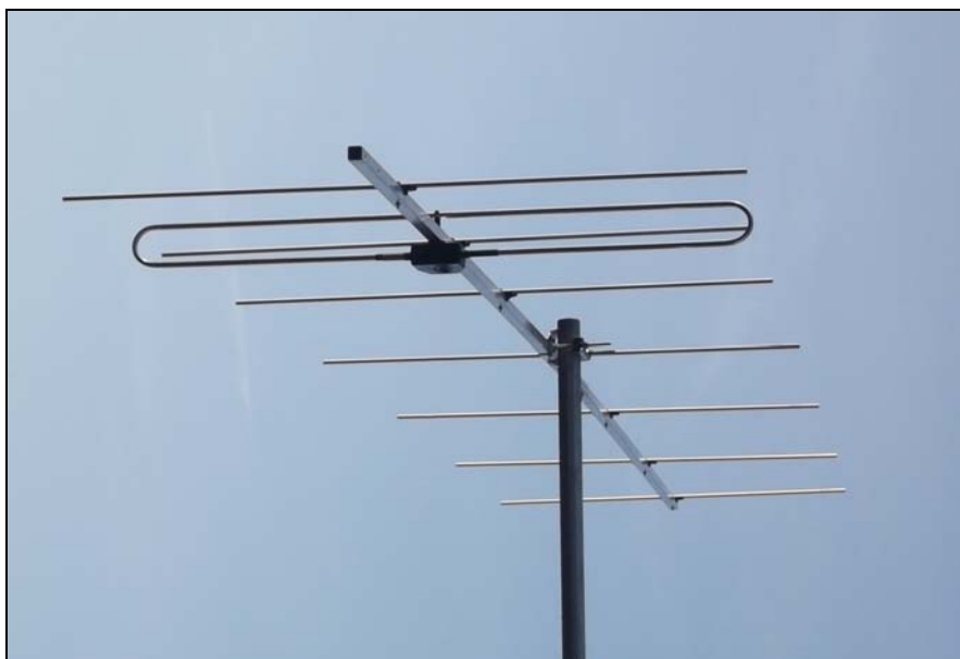
Fig. 7: 5-8 as 8 ele. version with folded DE
