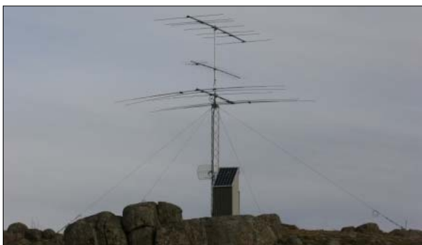
Fig. 9 & 10: VK3OE's remote site, thus VK3OER, is an internet connected (3G and microwave to DSL) remote site using solar power. The remote rig units are used to provide connection (see remoterig.com). The site is at 570m and has a clear take off in all directions well below 0 degrees except in the direction of Mt Alexander where the horizon is at +1 degrees. Frequencies are 14 MHz, 21 MHz, 28 MHz, 50 MHz and 144 MHz. Left antennas, right take off to Europe.
