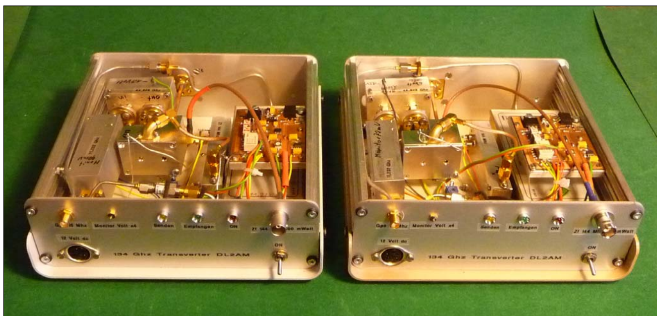
Fig. 7: Two 134 GHz transverters – ready for 2-way QSOs
