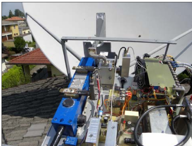
Pictures: Left: 24 GHz experimental feeds which allow for a greater gain on my offset dish compared to a W2IMU 1.8 wl – Middle: Picture B: Search for optimal opening on E and H plane and flare length of new feeds with WR42 WG – Right: 10 & 24 GHz Feeds. With the 10GHz feed installed on 2.7 m dish I measured 18 dB sun noise with SFU 135.7. I have calculated 50 dBi dish gain.
