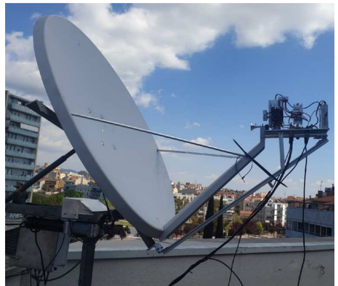
EA3HMJ's 47 GHz experimental EME station
