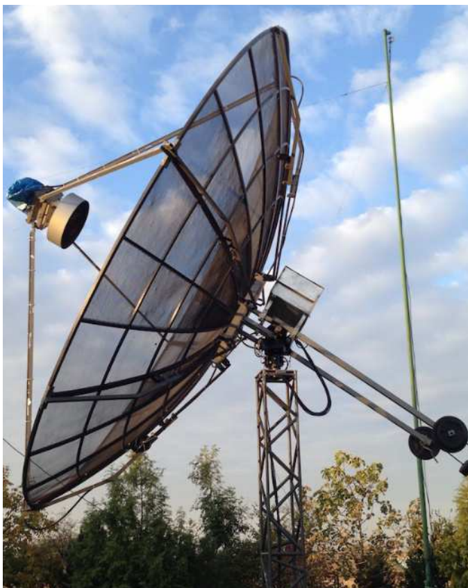
SP6ITF's 4.5 m dish used in 1296 Funtest
