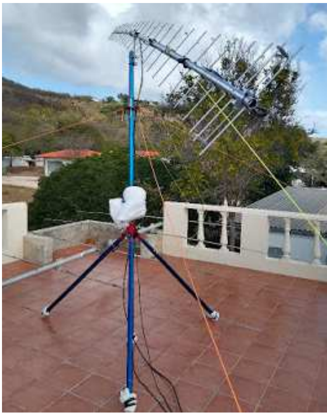
PJ2T's yagi at 45 deg pol angle seems to add +3 dB to EU
