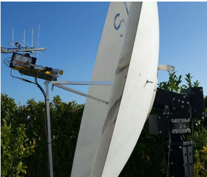
CT1BYM dish with 24 GHz feed in place
