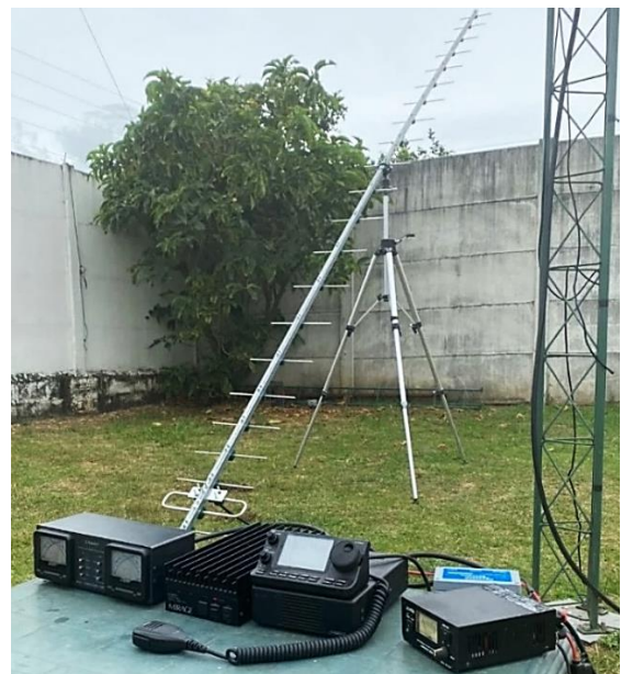
TI5CDA operated 432 in EME Contest with 22 el HB LFA yagi and 100 W
