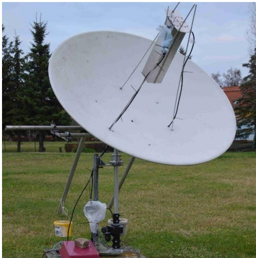
DL7APV's 1.8 m dish used on 1296 during the Contest
