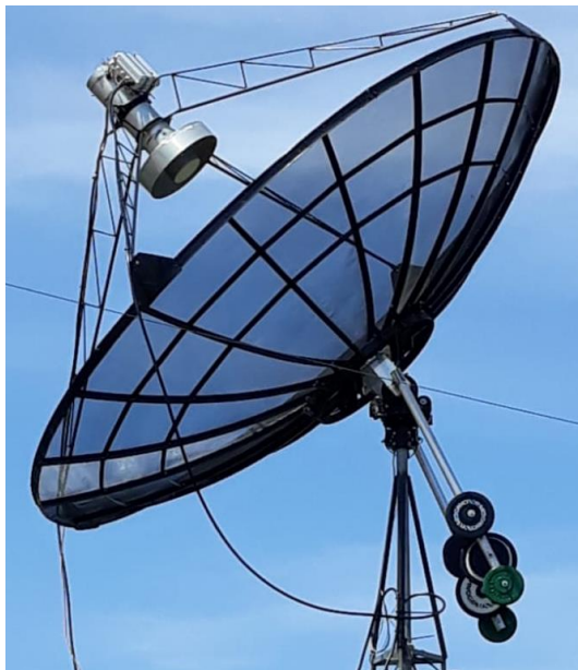
IK2DDR's 3.7 m dish used on 1296 in the contest
