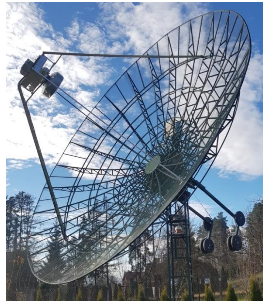
SP9VFD's newly constructed 6.4 m dish used on 1296
