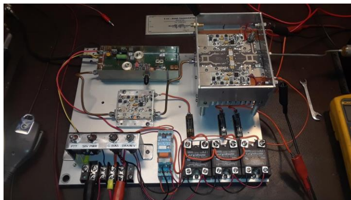
VE6BGT's 6 cm system and feed below – all HB
