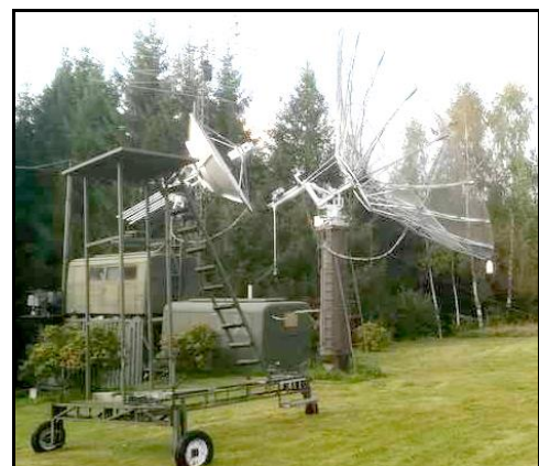
SP6OPN used a 6.5 m dish on 13 cm and SP6JLW used a 4 m dish for 3 cm
