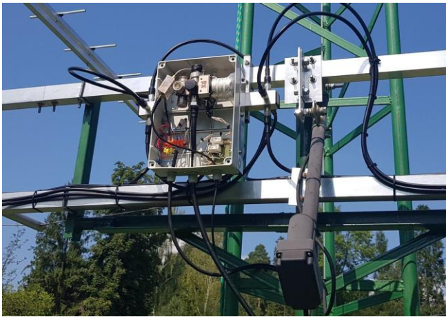
SP9VFD's 70 cm LNA box
