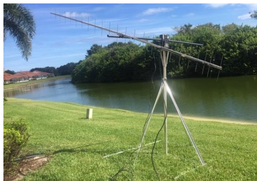
K1RS's yagi that he will use in the contest on 70 cm
