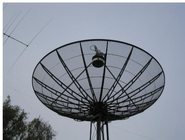
Fig.34 ON4BCB's feed for 1296 MHz
