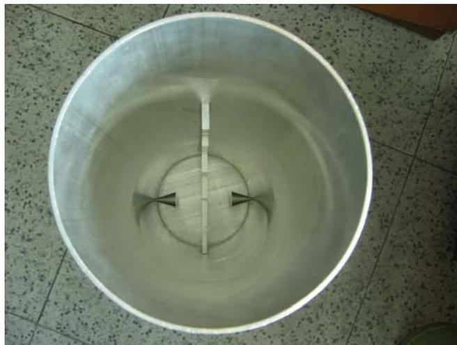
Fig. 6 Dural tube with probes and septum
