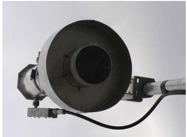
Fig. 32 OK1CA `s feed for 2300 MHz
