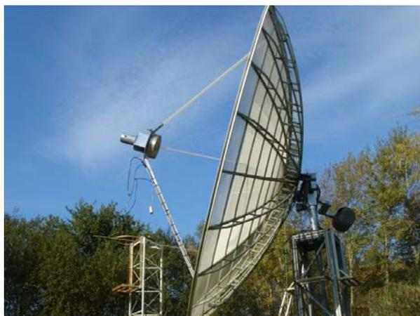
Fig 33b ON7UN's feed and sun noise measurement
