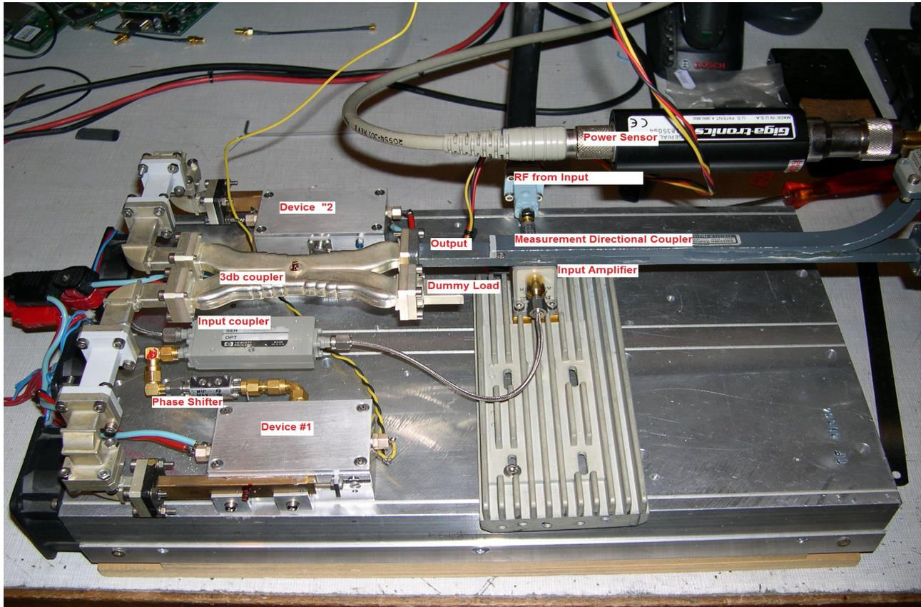
The reasonable performances achieved are more than 15 Watts (41.5 dBm) at the saturation, for approximately 340 mW (~25 dBm) at the input. Each TGA needs 21 to 22 dBm in, plus the insertion losses in each input branch which are around 2.5db (insertion loss is in addition to 3 dB coupling loss).
