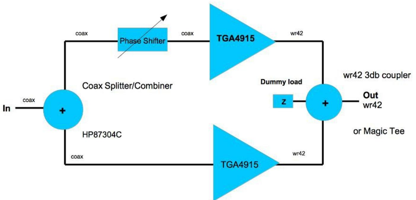
As a 26GHz phase shifter couldn't be found I used a 18GHz one; as it is a passive component, it is working fine at 24GHz except it has a little bit more losses. It's not a real problem if at the input you have enough dBm to drive the TGAs.
