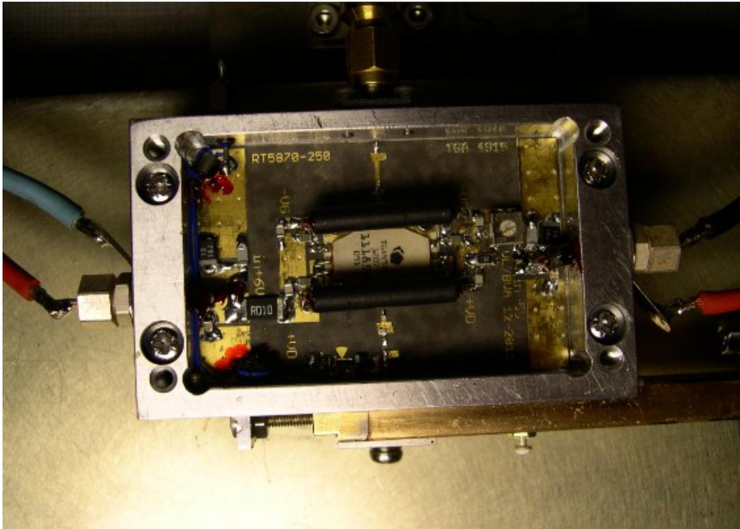
I could obtain 8+ Watts at the saturation, this is better than the specs announced and has been verified on my 3 units.
