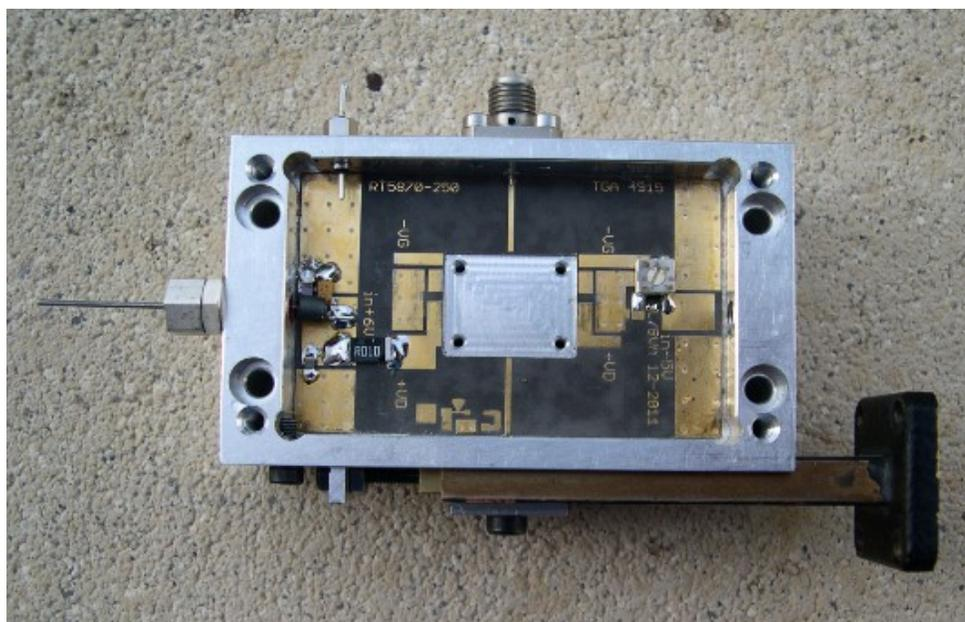
The mechanical drawings of the milled box are provided on the DVD so if you have your own milling machine tool or access to a numerical machine you could reproduce it quite easily.
