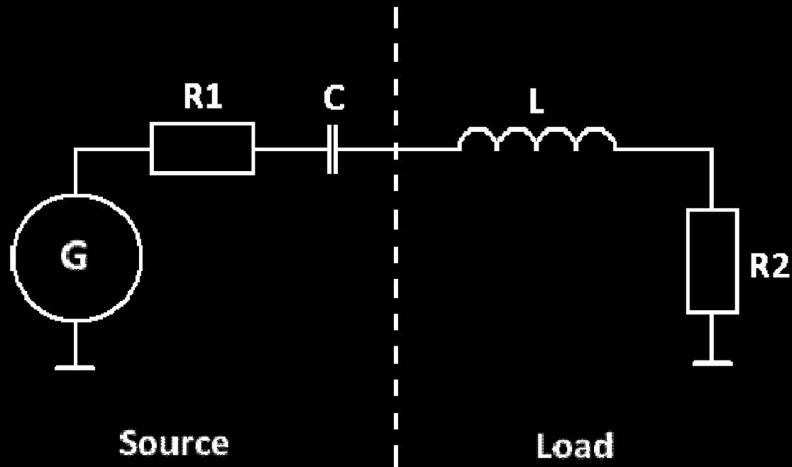
Basic utility focused for RF matching between source and the load
