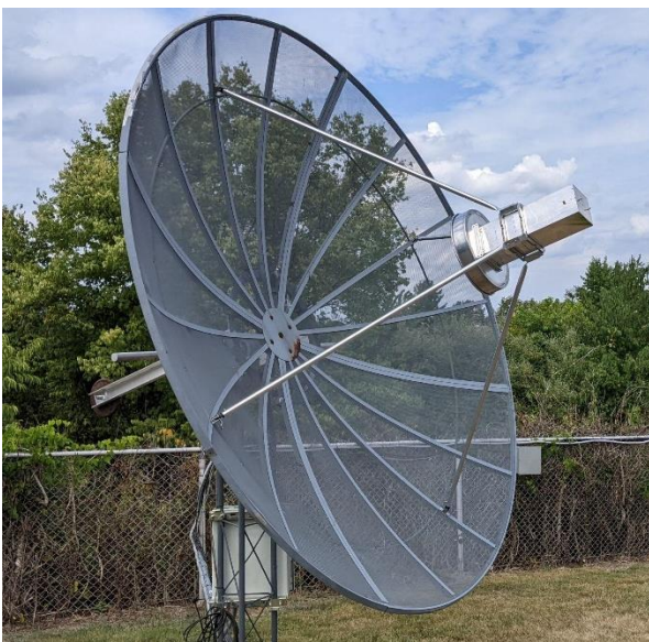
W2ZQ 3 m dish used on 1296 in the ARRL Contest
