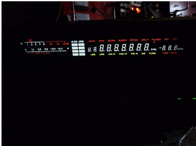
Searching at the internet I could find several articles which are reporting about problems with the "digital unit" but it seems that all problems could be removed if the backup battery is changed and the PCB in the neighbourhood of the battery is cleaned. Another problem at this radio seems are the electrolytic capacitors which getting leak.
